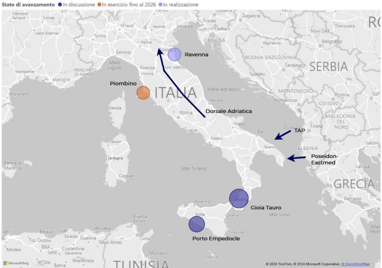
Figure 2 – New investments in gas infrastructure capacity in Italy either in progress or under examination (for the TAP, reference is made to an increase in import capacity of up to 10 bcm/year; transfer of the FSRU from Piombino to Vado Ligure is currently awaiting authorisation)
