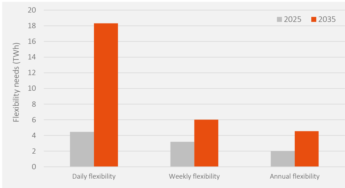
Figure 19 Evolution of daily, weekly and annual flexibility needs within Italy (TWh/year) 12 . Source: Artelys modelling.
