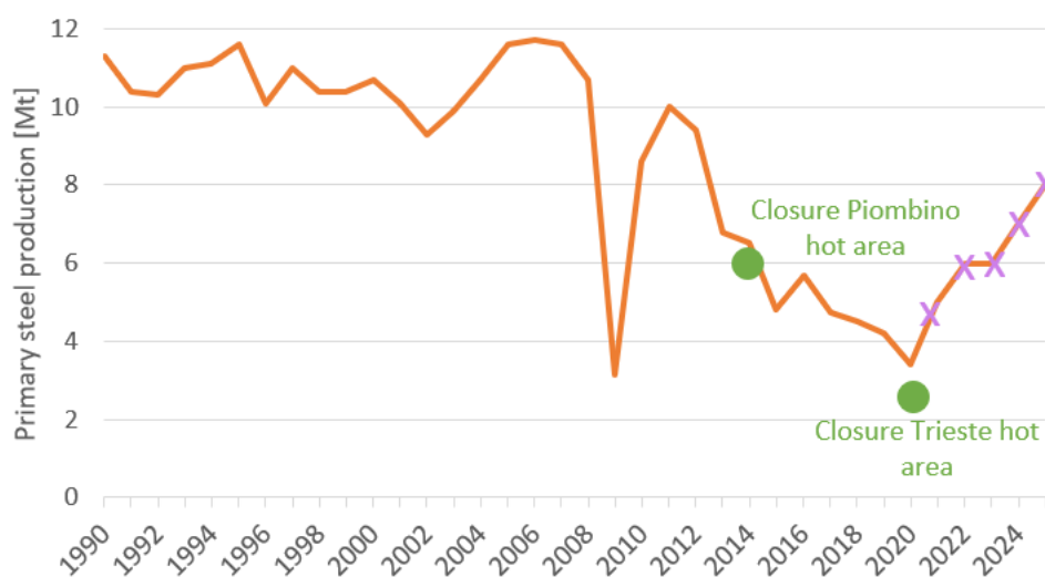
Figure 7 - Trend of primary steel production in Italy since 1990. Shown in purple is the 2021 - 2025 production level of the Taranto plant agreed between Invitalia and ArcelorMittal 30 .
